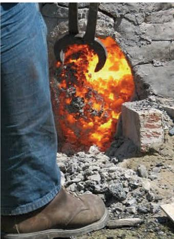
The local ore here in Northern California is magnetite sand, which is too rich in iron and too fine in size to run through the furnace like the bog ores that were commonly used in Scandinavia, so we mix it with silica sand and a binder to make pellets.
